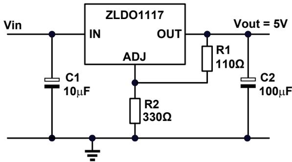
Figure 1 Basic Adjustable Regulator with 5V Output
