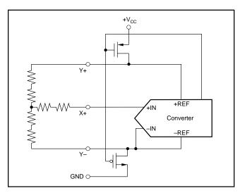
FIGURE 4. Simplified Diagram of Differential Reference (SER/ DFR LOW, Y Switches Enabled, X+ is Analog Input).
