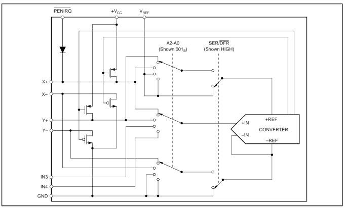
FIGURE 2. Simplified Diagram of Analog Input.
