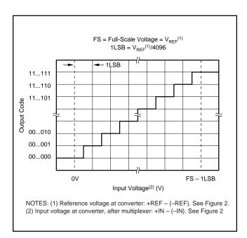
FIGURE 8. Ideal Input Voltages and Output Codes.
