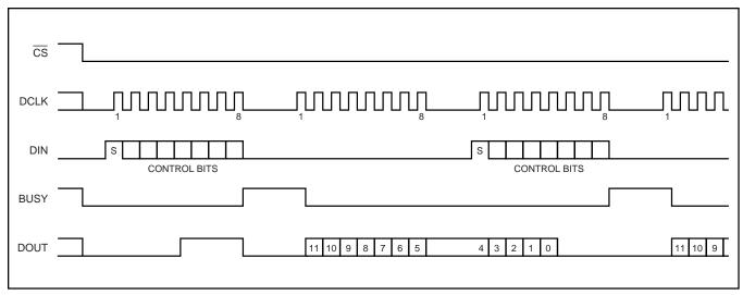
FIGURE 6. Conversion Timing, 16 Clocks per Conversion, 8-bit Bus Interface. No DCLK Delay Required with Dedicated Serial Port.
