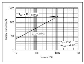
FIGURE 9. Supply Current versus Directly Scaling the Frequency of DCLK with Sample Rate or Keeping DCLK at the Maximum Possible Frequency.
