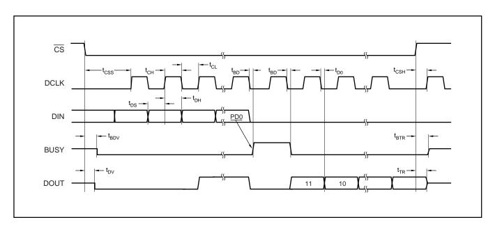
FIGURE 7. Detailed Timing Diagram.
