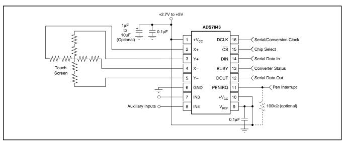
FIGURE 1. Basic Operation of the ADS7843.
