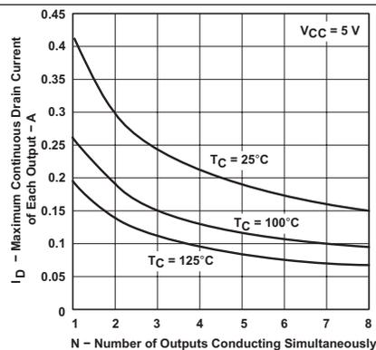
Figure 6. Maximum Continuous Drain Current of Each Output vs Number of Outputs Conducting Simultaneously
