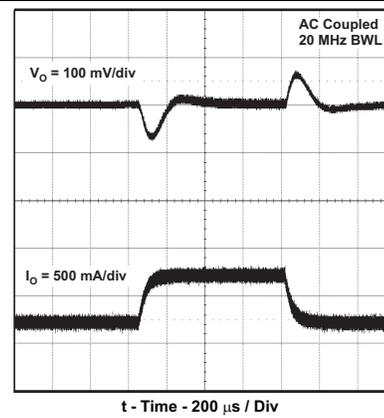
Figure 24. Transient Response,  $I_O$  Step 0.25 to 0.75 A
