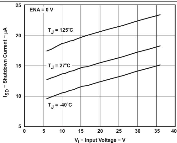
**Figure 7. Shutdown Quiescent Current vs Input Voltage**
