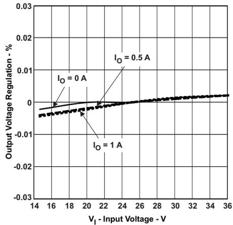
Figure 21. Output Voltage Regulation % vs. Input Voltage
