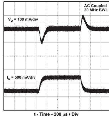
Figure 15. Transient Response,  $I_O$  Step 0.25 to 0.75 A
