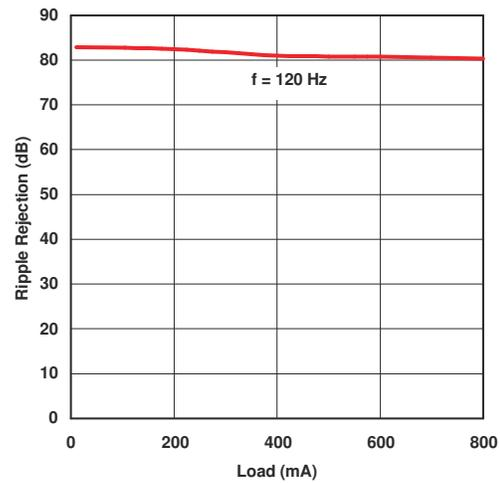
Figure 6-4. Ripple Rejection vs Load Current (ADJ Version)
