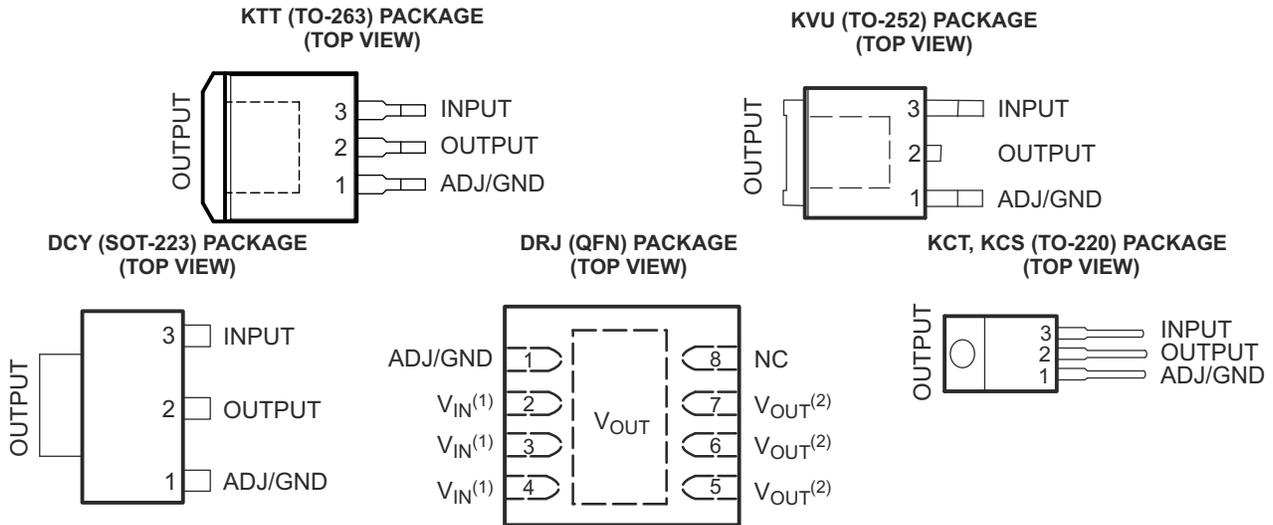
(1)  $V_{IN}$  pins (2, 3, 4) must be connected together.
