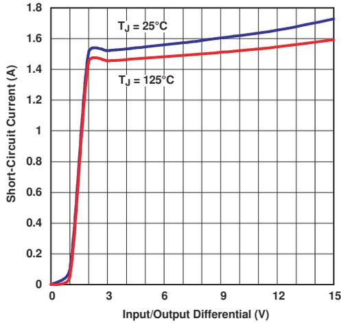
Figure 6-1. Short-Circuit Current vs ( $V_{IN} - V_{OUT}$ )
