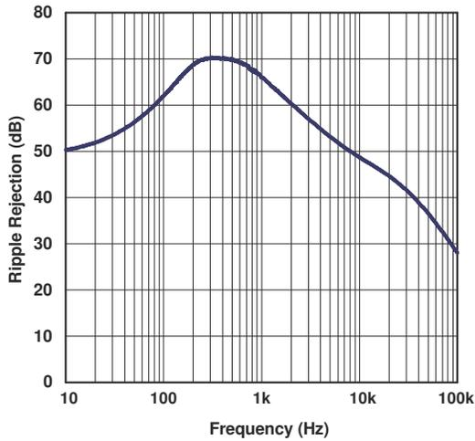
Figure 6-3. Ripple Rejection vs Frequency (ADJ Version)
