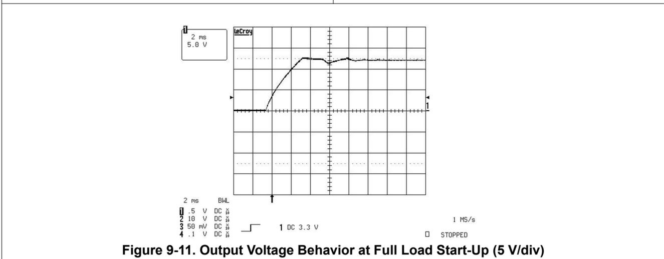
**Figure 9-11. Output Voltage Behavior at Full Load Start-Up (5 V/div)**
