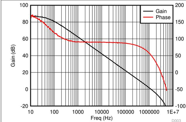
**Figure 7-3. Error Amplifier Open-Loop Gain and Phase vs Frequency, VCC = 15 V, R<sub>L</sub> = 100 kΩ, and T<sub>A</sub> = 25 °C**
