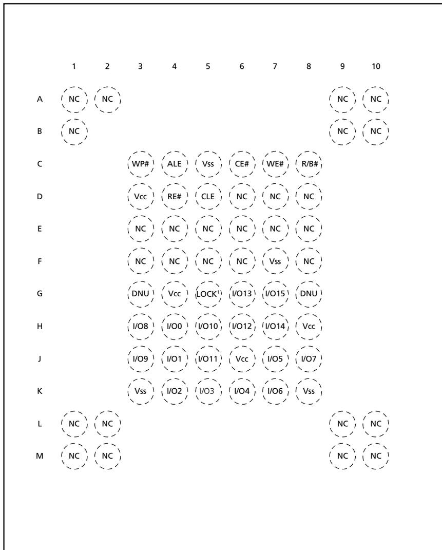
Note: 1. For the 3V device, G5 changes to DNU. NO LOCK function is available on the 3.3V device.
