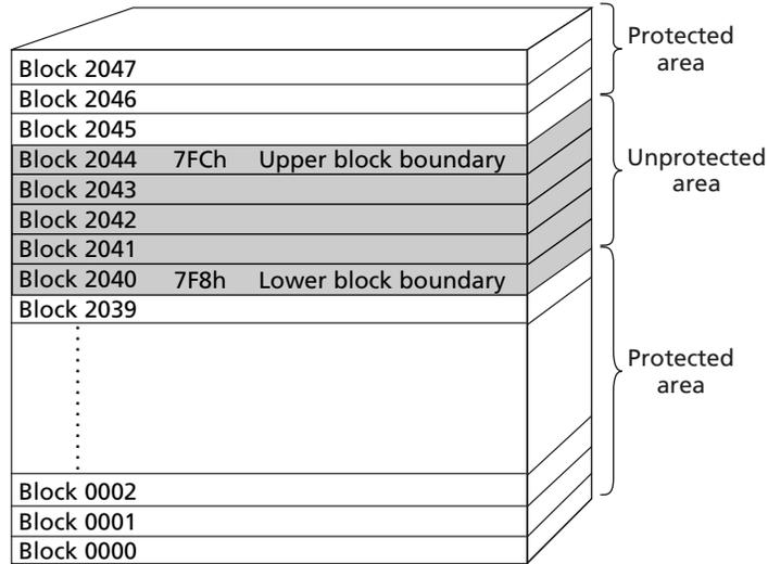
Figure 56: Flash Array Protected: Invert Area Bit = 1
