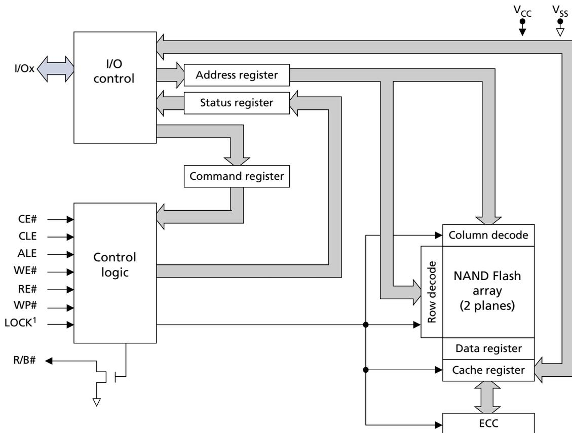
Note: 1. The LOCK pin is used on the 1.8V device.
